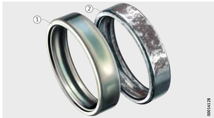
Figure 11 Bearing rings after the salt spray test
