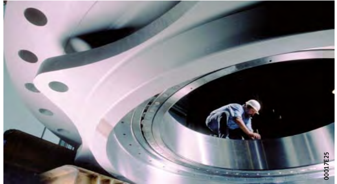
Figure 5 Mounting of a large rolling bearing
