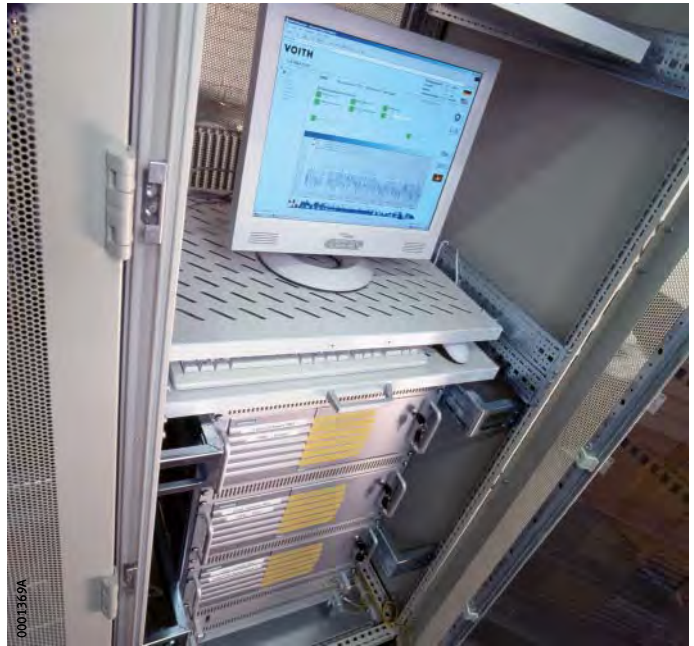
Figure 10 Condition-based rolling bearing monitoring using FAG VibroCheck
