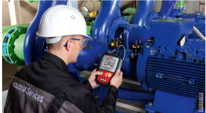
Figure 3 Shaft alignment device Top-Laser EQUILIGN
