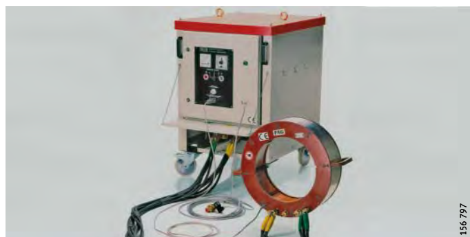
Figure 10 Induction heating device
